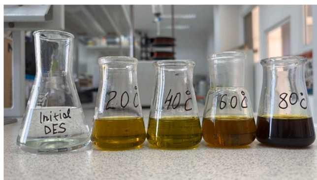
Fig. 7. Photographic comparison of DES leachates after magnetic fraction leaching at various temperatures.
